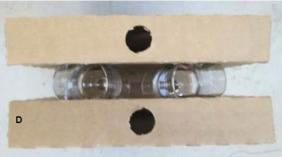
\*Difference between internal dividers with horizontal fluting (correct) and vertical fluting (wrong)
